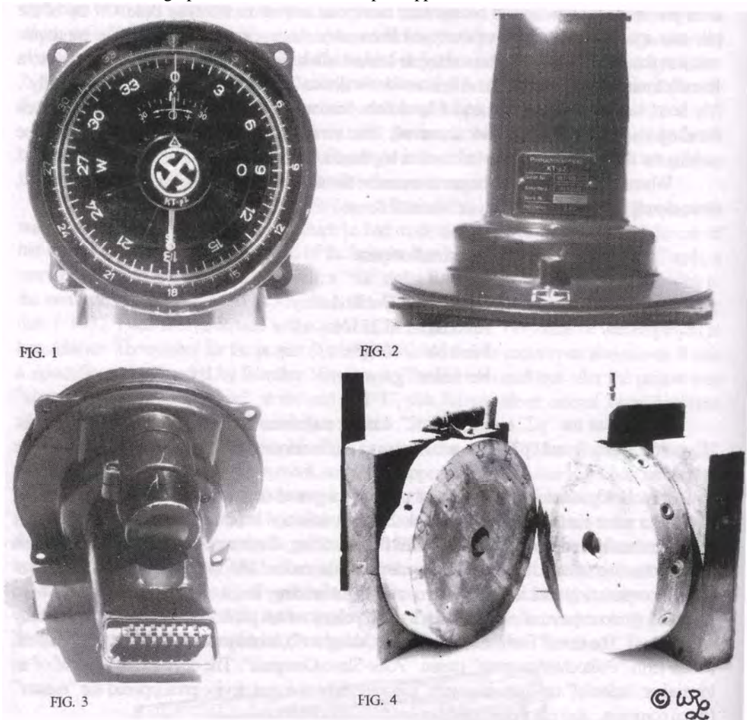
FIG. 1: Top View - fluorescent dial and face calibrations, with 12 30-degree peripheral increments. With master gyrocompass calibrated to true north prior to takeoff directional selections made with dial read on Peiltochterkompass.
